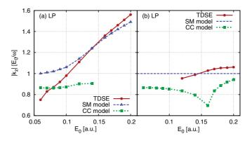
FIG. 4. (Color online) Position of the maximum in the (a) longitudinal distribution  $P^{\text{LP}}(k_z)$  and (b) lateral width  $\sigma^{\text{LP}}(k_z)$ , plotted versus field amplitude for the LP pulse.
