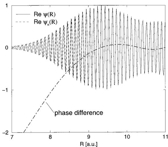
FIG. 5. Real part of the exact (full line) and iterated (dashed line) wave function obtained in the case that the input momentum density is measured with a limited resolution. Also shown is the phase difference between the two functions.
