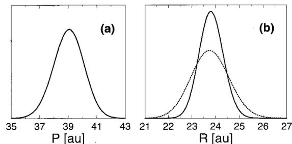
FIG. 6. (a) Momentum-space densities for fragments obtained after femtosecond excitation of  $I_2$  molecules into the  $B$ -state dissociation continuum (laser pulse width: 125 fs). Here the case of excitation with an up-chirped or a down-chirped pulse result in almost identical distributions. (b) Coordinate-space densities for up-chirp (solid line) and down-chirp (dotted line) excitation.
