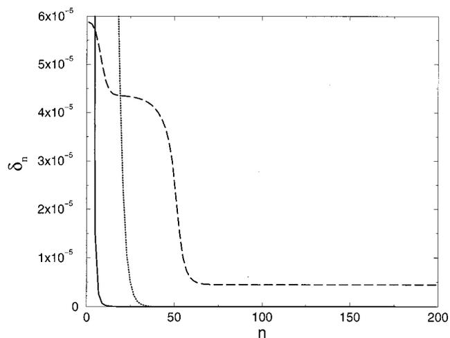
FIG. 7. Convergence behavior of the Gerchberg–Saxton algorithm. Shown is the mean deviation of the iterated coordinate-space amplitude from the exact one, as defined in Eq. (16). Solid and dashed line: Up-chirp excitation; dotted line: Down-chirp excitation. Depending on the initial condition, the deviation tends to zero (convergence and phase retrieval) or a constant (no convergence), see text.
