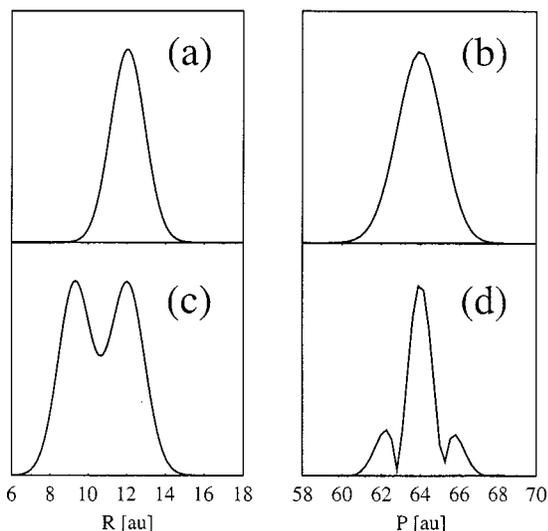
FIG. 2. Modulus of the coordinate-space (a) and momentum-space (b) wave function resulting from the interaction with a 30 fs pump pulse. (c) and (d): Same as (a) and (b) but for a pump pulse consisting of two 30 fs pulses which are time-delayed by 40 fs.
