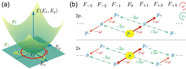
FIG. 1. (a) Energy surfaces of the 2p states for  $\text{Ne}^+$  in an electric field and paths of the electric field in the parameter space for CP (red) and 1:1 bicircular (yellow) fields. (b) Illustration of the possible transitions in the bicircular field.
