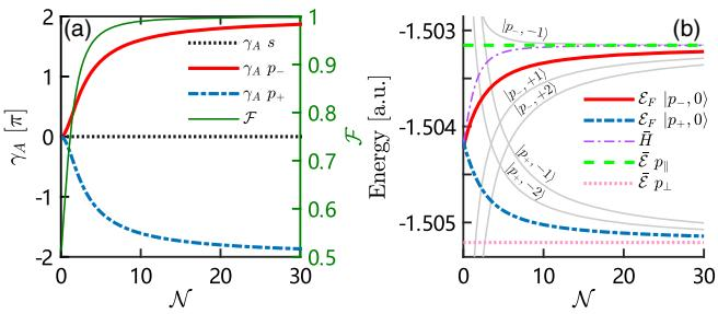
FIG. 2. Results for a CP field with intensity  $5 \times 10^{14}$  W/cm<sup>2</sup>. (a) AA phases  $\gamma_A$  and adiabaticity indicator  $\mathcal{F}$  for p-type states. (b) Energy curves.  $|p_{-}, 0\rangle$  denotes a solution for  $|P(t)\rangle$  that resembles the  $p_{-}$  state at the smallest considered  $\mathcal{N}$ , while  $|p_{-}, n\rangle$  denotes a solution with quasienergy differing by  $-n\omega$ .
